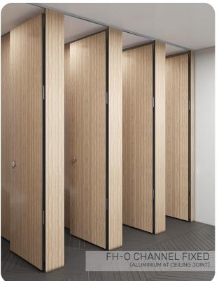
The FH Full Height partition system is the perfect system for complete cubicle privacy. The FH system has floor to ceiling panels and doors with clearances of 20mm FFL and 55mm FCL. The 55mm clearance at the top of the doors allows the lift off hinges to function in case of emergency. The FH partition system is the next best thing to an individual room but at a fraction of the cost.
